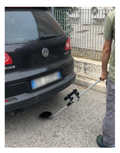
Efis 1 is a mirror mounted on a telescopic rod to perform subvehicular checks in areas particularly at risk. In areas with high vehicle flow, Efis 1 allows quick inspections, even in low light conditions thanks to the supplied torch. Incredibly light and waterproof, it is a ready-to-use safety device.
